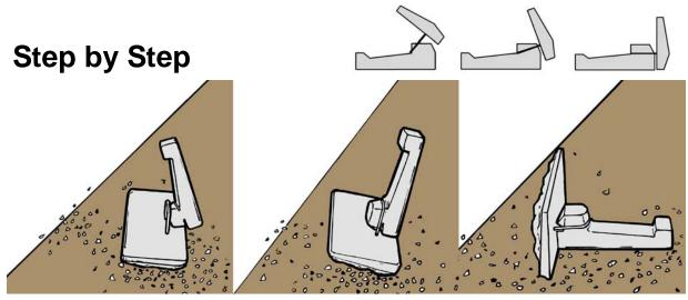
**Retaining Module Assembly**
